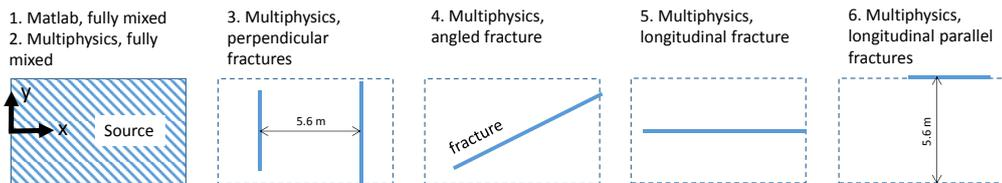
**Figure 19. Representation of the scenarios. the source and fractures are shown on a plane corresponding the top of the aquifer (the x direction is the groundwater flow direction). The total length of the fractures in each scenario is the same in order to have the same contaminant mass discharge in all scenarios.**
