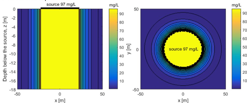
**Figure 28. pce concentration in a vertical cross section ( $y=0$  M) (left). Pce concentration at the top of the aquifer in plan view (right); the black dashed line shows the location of the contaminant source. model IV.**
