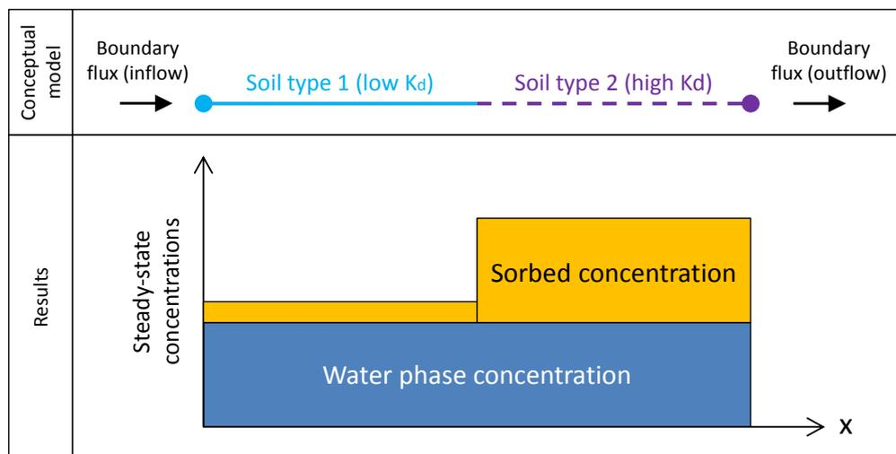
**FIGURE 31. (TOP) CONCEPTUAL MODEL A HORIZONTAL CONTAMINANT FLUX ENTER THE SOIL TYPE 1 FROM THE LEFT END, IT CROSSES BOTH THE 2 SOIL TYPES AND THEN IT OUTFLOWS THROUGH THE RIGHT BOUNDARY. (BOTTOM) RESULTS. THE WATER PHASE CONCENTRATION IS THE SAME IN THE 2 SOIL TYPES, HOWEVER THE SORBED CONCENTRATIONS ARE HIGHER IN SOIL TYPE 2 WHICH HAS A HIGHER DISTRIBUTION COEFFICIENT  $K_d$ .**
