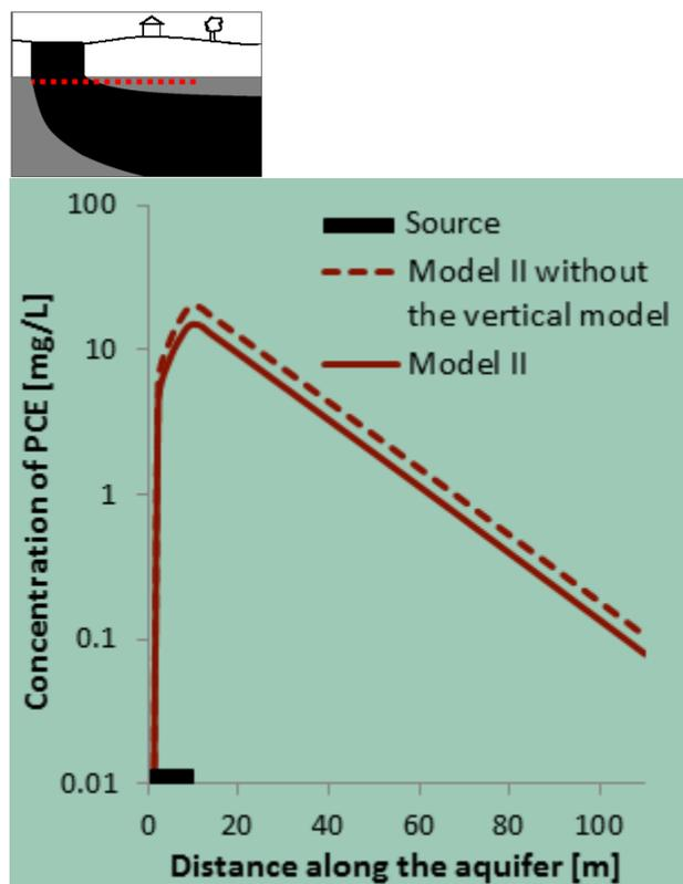
Figure 17. Concentration of PCE in the aquifer (there are fully mixed conditions in the aquifer, a 2d solution is used so there is no variation in concentrations in the  $z$  direction).  $I=82$  MM/Y. Note that concentrations along  $y$ -axis are log-scale.
