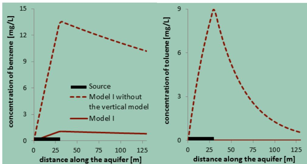
**Figure 14. Concentration of benzene and toluene in the aquifer. The aquifer is thin and so is fully mixed in the vertical direction and so the 2d solution is used.  $I=300 \text{ MM/Y}$**
