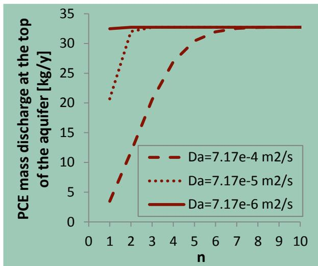
Figure 27. PCE total mass discharge at the top of the aquifer at MW Gjøes vej as a function of different integration intervals  $N^*[\text{MAX}(\text{LX}, \text{LY})]$  and Different air diffusion coefficients,  $dA$ .
