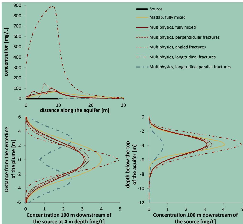
**Figure 20. Concentration in the aquifer as a function of different fracture geometries. (A) concentrations along the x-axes and at 0.01 M DISTANCE FROM THE TOP OF THE AQUIFER. (B) concentrations as a function of the distance below the top of the aquifer 100 M downstream the source. (C) concentrations as a function of distance from the centerline of the plume at a depth of 4 M below the top of the aquifer and 100 M DOWNSTREAM THE SOURCE.**
