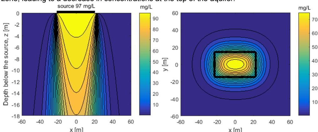
**Figure 22.** Concentration in a vertical cross section below the source ( $y=0$  M) (left). Pce concentration at the top of the aquifer in plan view (right) ( $z_v=18$  M); the black line shows the location of the contaminant source.
