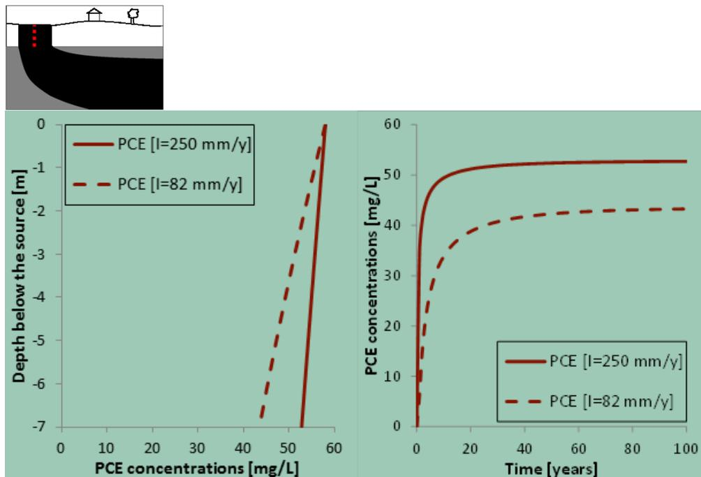
**Figure 16.** Concentration of PCE as a function of the depth below the source and the different recharge rates  $I$ . (left). the level -7 M corresponds to the top of the aquifer. Concentration of PCE as a function of time (using the model DTU v1d of Chambon et al., 2011) at 7m depth (right).
