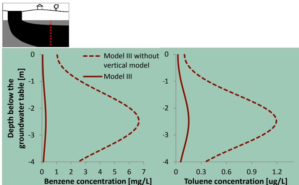
Figure 26. Model III application to easy degradable compounds. concentrations of benzene and toluene in the aquifer.
