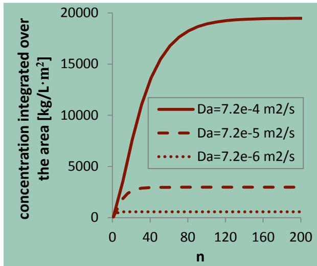
Figure 30. Concentration at the top of the aquifer at MW Gjøes vej as a function of different integration intervals  $N \cdot \text{RADIUS}$  and different air diffusion coefficients,  $dA$ .
