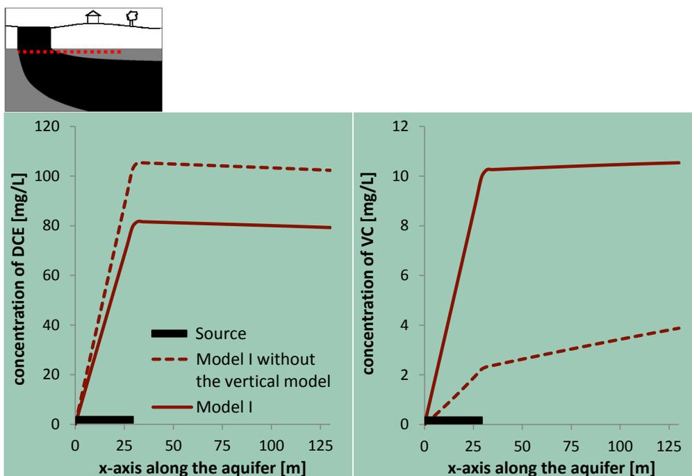
Figure 12. concentration of DCE (left) and VC (right) in the aquifer (note that there are fully mixed conditions in the thin aquifer so there is no variation in concentrations in the  $z$  direction).  $I=300 \text{ MM/Y}$ .
