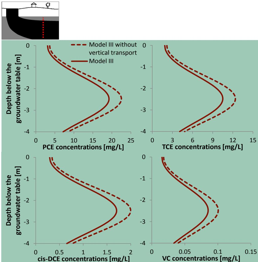
Figure 24. Contaminant concentrations 100 M downstream the source ( $100 \text{ M} + L_x/2$ ) as a function of the depth below the groundwater table. concentrations are calculated using both model III and Model III without vertical transport.
