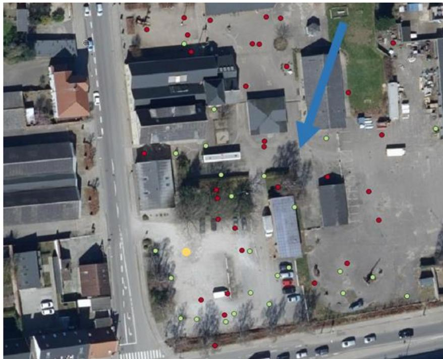
**Figure 1.** Map of the former gasification plant in Horsens. The red and green dots represent previous drillings, where red dots represent closed and unavailable drill holes and green dots represents drill holes conserved, and available for further studying. The yellow dot shows the location of the drill hole B404, in which samples was collected. The blue arrow indicates the direction of the groundwater flow.
