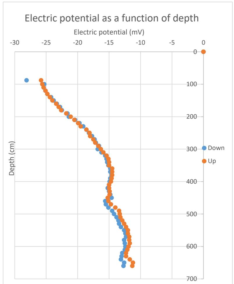
**Figure 2.** EP measurements every 10 cm down drill hole B404. Blue dots represent measurements from lowering the electrode down the drill hole, and orange dots represent measurements from raising the electrode up the drill hole.
