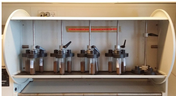
Figure 2. The photograph shows the extraction carried out in 50 ml polypropylene tubes in a “head over end” rotary shaker for 24 hours.
