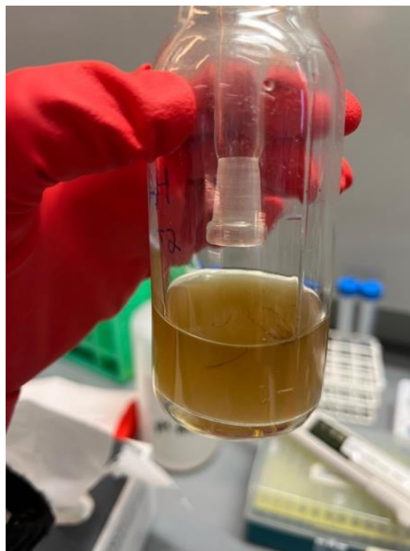
Figure 4: Image showing darkening of media and presence of substance likely to be pyrogallol
