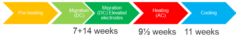
Figure 8.1: Overview of conducted stages and durations. Note that the electrodes were raised after 7 weeks of the DC migration stage and stayed elevated through the rest of the pilot test.
